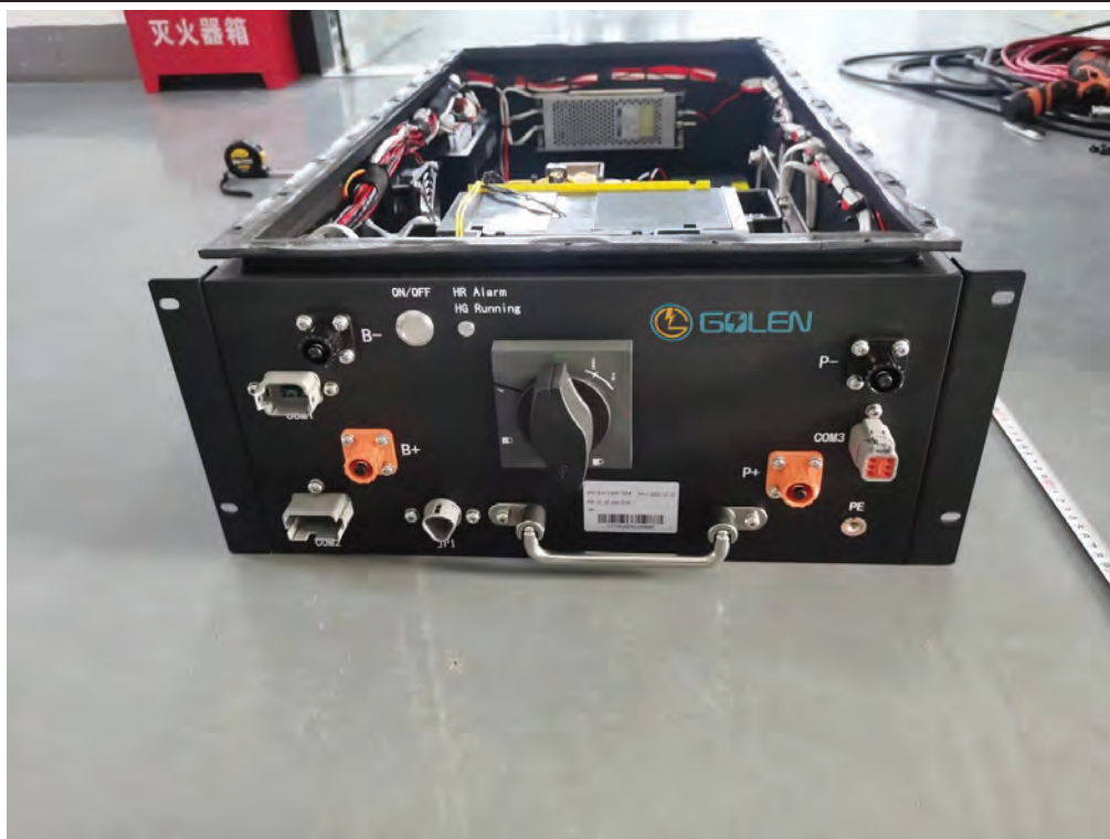
Internal and terminal view - Battery Pack
